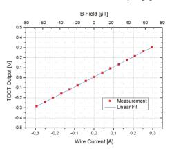
Figure 2: Stretched wire measurement with TMR-sensor MMLP57FD, note the good linear response.
