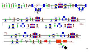
Figure 1: Schematic layout of CBPMs in the undulator section.
