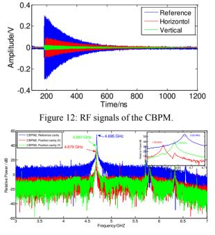
Figure 13: Frequency spectrum of the CBPM.
