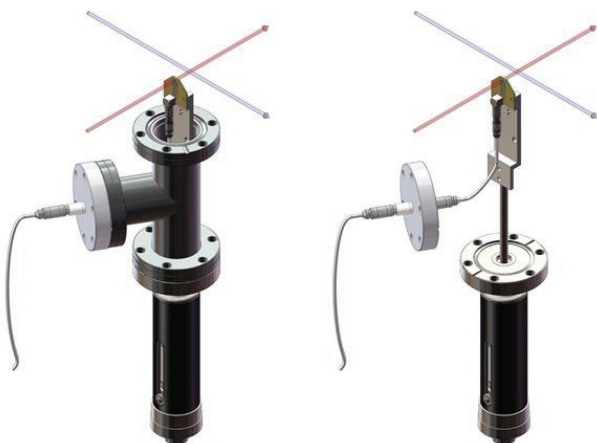
Figure 6: CAD rendering of the THz detector PCB mounted on a retractable mechanical feedthrough to bring the chip near the electron beam (blue arrow). The probe laser (red arrow) enters the vacuum chamber through a viewport (not shown). With the tee suppressed (right), the triaxial signal coupling can be seen.
