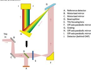
Figure 2: Preliminary broadband spectrometer design for beam length measurements. The linear polarizer is not shown.
