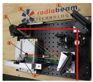
Figure 1: Physical layout of final spectrometer design, shown with dimensions and optical path
