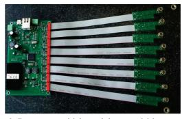
Figure 3: Prototype multichannel data acquisition system.
