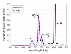
Figure 2: Typical spectrum from the Doppler system showing the Balmer  $\alpha$  ray and Doppler shifted rays of H, H<sub>2</sub> and H<sub>3</sub>. The vertical lines are positioned using the Doppler shift equation, the mass and energy of the species, and the geometrical angle of observation.
