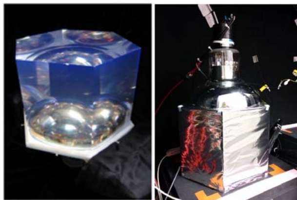
Figure 2: SuperNEMO OM, showing bare plastic scintillator block (left) and wrapped block with PMT (right).
