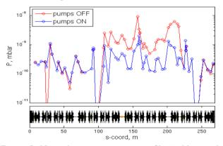
Figure 5: Normal vacuum pressure profile (in blue, with pumps on), compared with the pressure profile (red trace) when the pumps in Sectors S07 - S13 are switched off.
