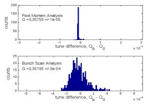
Figure 4: Bunch-by-bunch tune using the Post Mortem Analysis (top) and the Bunch Scan Method (bottom).
