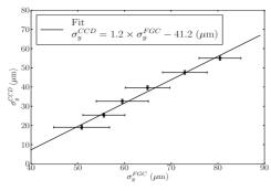
Figure 2: Resulting beam size, measured by the FGC for different couplings versus the same measurement done with a standard CCD.
