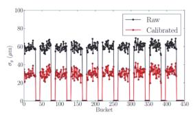
Figure 3: Measured BbB beam size with the ALBA filling pattern: 10 trains, with 32 bunches/train spaced by 12 empty buckets. The final gap is larger (20 buckets).
