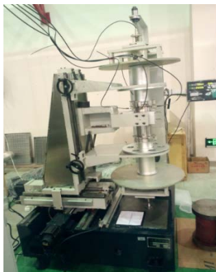
Figure 5: Automatic BPM Calibration System.
