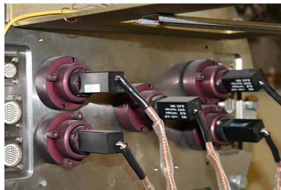
Figure 8: Photomultipliers for scintillators based detectors.
