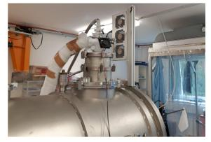
Figure 8: The cryomodule of Gun III during cooling with liquid helium.
