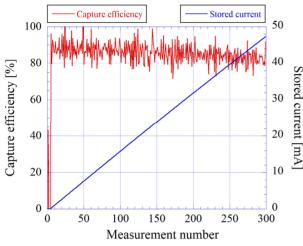
Figure 8: PF-AR capture efficiency measured by using the calibrated BPM and a DCCT for the ring.
