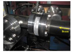
Figure 7: Photograph of the in-flange ICT installed near the exit of the new BT.
