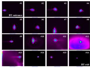
Figure 5: Injected beam profiles along the new BT measured by the SCMs. Data of the last SCM#17 are missing due to an insufficient adjustment of the camera optics.
