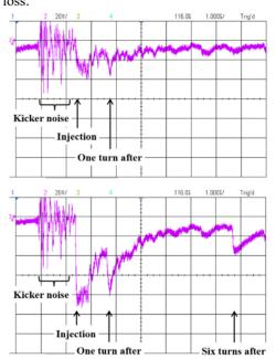
Figure 9: Turn-by-turn measurement of the injected beam loss using the BLM. Without (upper) and with (lower) inserted screens.
