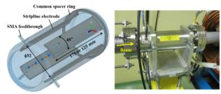
Figure 2: Schematic and photograph of the stripline BPM.
