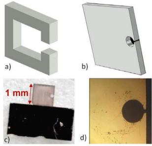
Figure 4: a) "Classical" SRR [5] with gap dimensions of 20  $\mu$ m (height) x 20  $\mu$ m (width) x 20  $\mu$ m (length), b) manufacturing design with increased gap length / plate thickness of 20  $\mu$ m x 20  $\mu$ m x 80  $\mu$ m, c) and d) images of the prototype SRR made from glass with gold coating.
