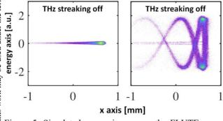
Figure 5: Simulated screen images on the FLUTE spectrometer showing the effect of 5 keV/c kick strength [7].
