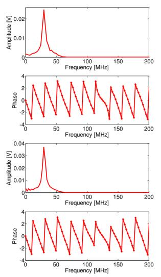
Figure 5: Magnitude spectrum and phase spectrum of two IF signal.
