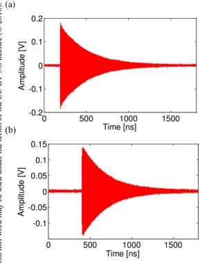
Figure 3: The raw RF signal for 200 pC bunch charge; a) port 3, b) port 1.
