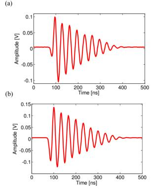
Figure 4: The raw IF signal for 200 pC bunch charge; a) port 1 and 3, b) port 2 and 4.
