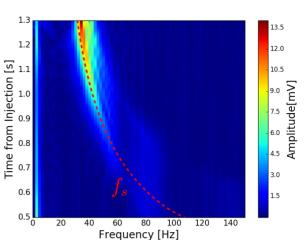
Figure 6: Spectrogram for the I component h=8 ( $I_8$ ). Red dotted line represents the estimated synchrotron frequency.
