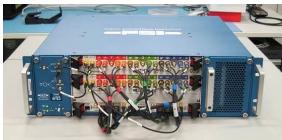
Figure 5: Modular BPM unit, with two cavity BPM RFFEs (top) and FPGA carrier board with two ADC mezzanines (bottom).
