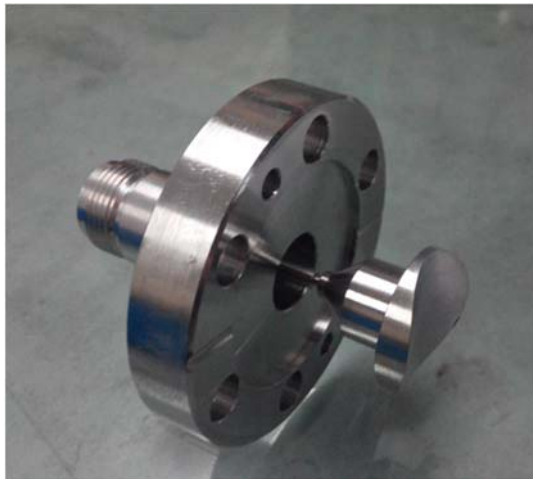
Figure 4: Removable feed through of cold BPM.
