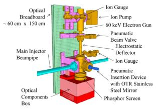
Figure 5: Model of the EBP showing the main components.
