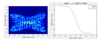
Figure 4: Simulated image of successive electron beam sweeps along the proton beam direction. The sweeps near the center are difficult to separate and may need to be split across multiple camera frames.
