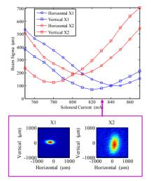
Figure 8: Horizontal and vertical rms beam sizes at the first (blue) and second (red) crosses in the test stand. The measurements are from OTR taken at  $\sim$ 50 keV and 1 mA beam current onto the stainless-steel mirrors.
