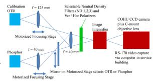
Figure 7: Conceptual layout of the optical paths followed by the OTR light and the phosphor screen light. Of the two lenses in each path, the second one is shared.
