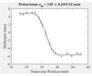
Figure 11: Electron beam deflection as a function of impact parameter with the proton beam. The uncertainties are just an estimate of how well one can determine the peak deflection from the images in Fig. 10.
