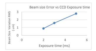
Figure 6: Relation between stability of the measured beam size and the CCD exposure time.
