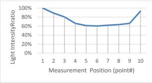
Figure 4: Intensity distribution of synchrotron light.
