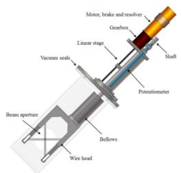
Figure 2: Simplified layout of the profile monitor.
