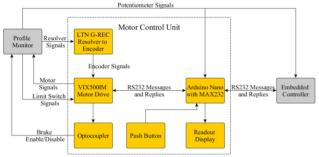
Figure 3: Block diagram of the motor control unit.
