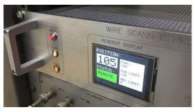
Figure 4: Motor control unit readout display.
