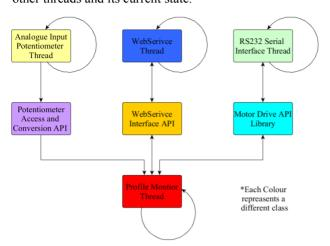
Figure 6: Software Architecture.
