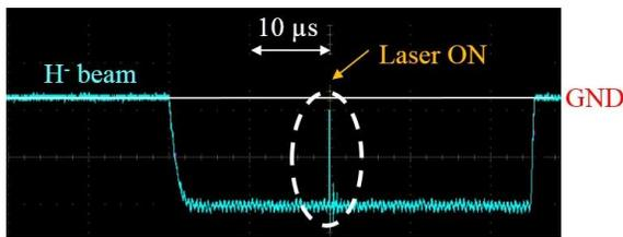
Figure 7: Current waveform of the H<sup>-</sup> beam observed at the 23° beam dump.
