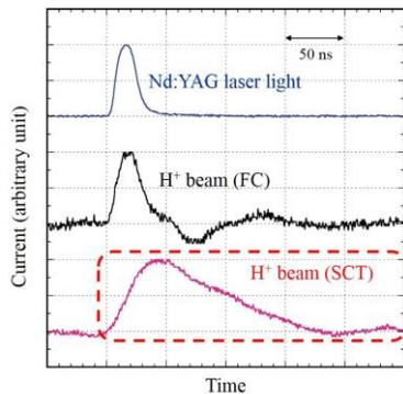
Figure 8: Current waveform of the H<sup>+</sup> beam observed at the 23° beam dump.
