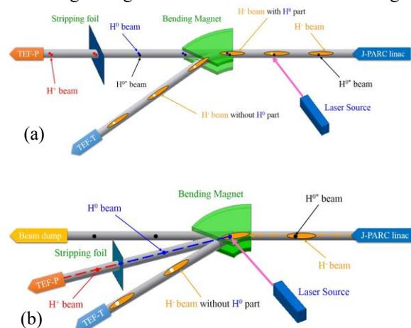
Figure 1: Conceptual diagram of the LCE device for TEF-P. For (a), the laser light is injected in the straight section of the  $H^-$  beam line. On the other hand, for (b), the laser light is injected in the bending section of the magnet. The neutralized proton due to interaction by the laser light is written as " $H^0$ ", and the pre-neutralized proton due to interaction by the remaining gas in accelerator tubes is written as " $H^{0*}$ ".
