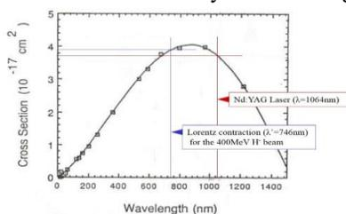
Figure 2: Cross section for  $H^-$  photoneutralization as a function of photon wavelength in the centre-of-mass frame [8]. The blue line shows the Lorentz contraction for the  $H^-$  beam with 400 MeV.
