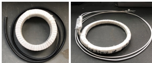
Figure 3: A 50-turn BCT and a 20-turn FCT fabricated in the BI lab of CSNS.
