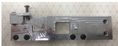
Figure 3: Tension testing apparatus to evaluate the tensile properties of BNNT thread using the wire-scanner leaf spring clamps.
