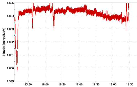
Figure 4: Electron beam kinetic energy during the same time period as Fig. 3.
