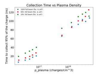
Figure 7: Time required to collect 95% of  $Q_{coll}(t\rightarrow\infty)$ , as a function of plasma density, for various detector biasing levels.
