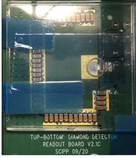
Figure 2: Full view of the readout PCB showing the AC return path provided by a highly parallelized array of 22 μF capacitors. Note that in this photograph, the assembly is rotated by 180 degrees relative to that of Fig. 1.
