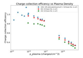
Figure 6: Estimated charge collection efficiency as a function of plasma density (cm<sup>-3</sup>) for 100 V, 60 V and 20 V sensor bias.
