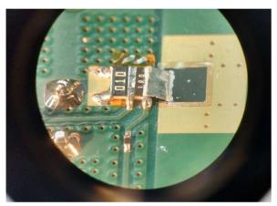
Figure 1: Detail of the readout PCB signal path showing the 37 µm thick diamond sensor, the low-impedance indium band connecting the sensor to the readout network, the series array of 1  $\Omega$  and 10 m $\Omega$  resistors that shunt the signal to ground, and the two 50  $\Omega$  pick-off traces.
