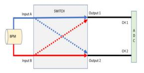
Figure 1: Switching Block Diagram.
