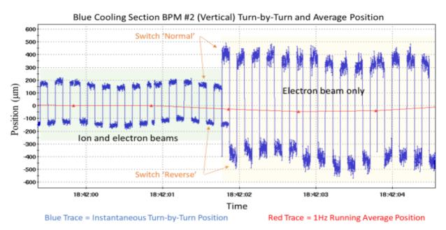
Figure 3: Calibration difference with ion and electron beam (left) vs. electron beam only (right).
