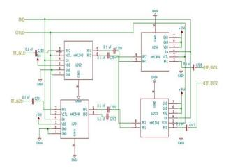
Figure 2: Switching Circuit Schematic.
