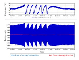
Figure 4: Drift over 24 hours due to temperature.
