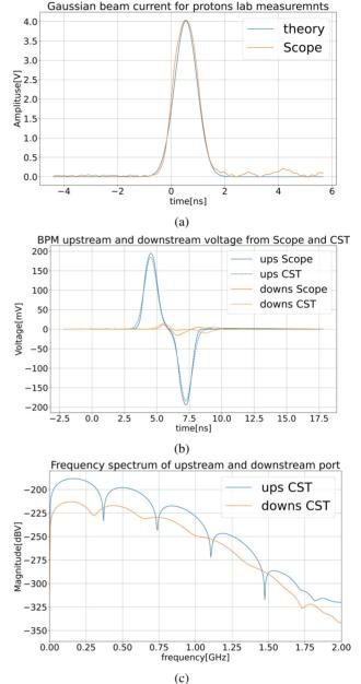
Figure 6: (a) Proton bunch signal, time-domain. (b) Stripline BPM response, TD, upstream and downstream ports (c) Stripline BPM response, FD, upstream and downstream ports.
