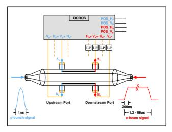
Figure 9: BPM measurement setup schematic.
