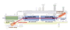
Figure 1: Sketch of the HL-LHC hollow electron lens (HEL).
