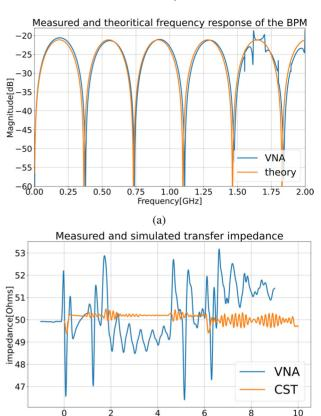
Figure 5: (a) The frequency response of the BPM stripline electrode, upstream port (S21) from measurement (VNA) and theory, and downstream port (S31). (b) Measured / simulated TDR of the BPM test bench setup.
