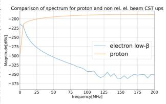
Figure 8: Frequency-domain magnitude spectrum for the low-beta electron beam signal, and the residual proton beam error signal.
