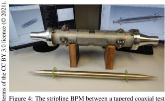
Figure 4: The stripline BPM between a tapered coaxial test bench structure with the inner and outer conductor.
