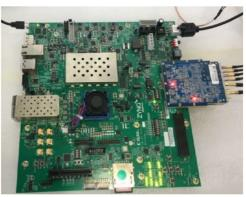
Figure 5: Photo of data acquisition board.
