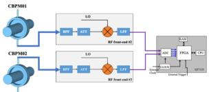
Figure 11: The scheme of measuring the bunch arrival time and bunch flight time.
