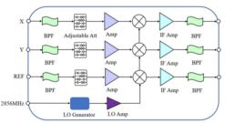
Figure 3: Schematic diagram of the RF front-end.
