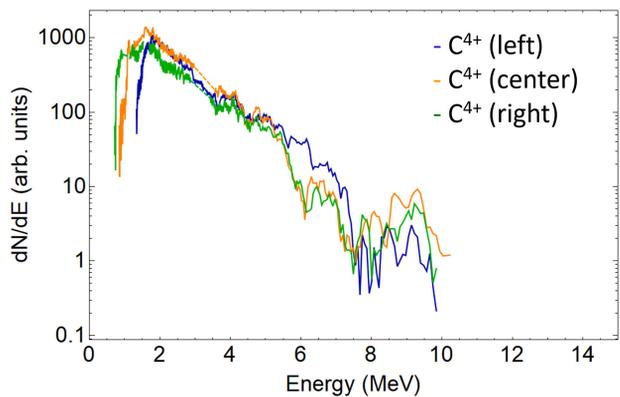
Figure 5: Left, center and right  $C^{4+}$  beamlets spectra from traces of Fig. 2.
