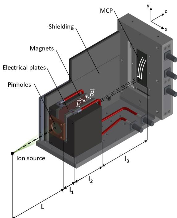
Figure 1: Multi-pinhole TP spectrometer design.
