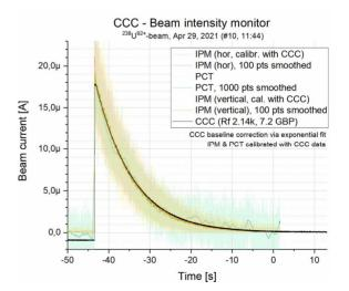
Figure 4: CCC current measurement compared to IPM and PCT in CRYRING. Rf = Feedback resistor value, GBP = Gain Bandwidth Product of the SOUID electronics [9].
