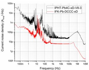
Figure 8: Comparison of current noise from an advanced axial CCC prototype (black) and a dual core CCC (red) at XD-dimensions (outer diameter: 350 mm).
