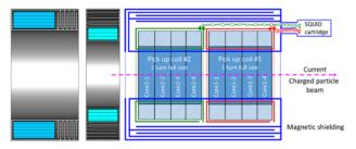
Figure 2: Magnetic shieldings with radial (left) and axial (middle) meanders. The ring-core of the radial CCC is indicated in blue, the detector volume of the axial CCC in turquois. Right: Schematic sectional view of the DCCC with axial meanders and two independent, fourfold segmented (due to material width limitations) toroidal cores.
