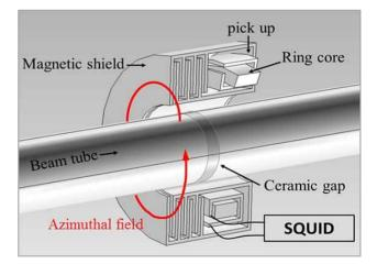
Figure 1: Classical CCC, shielding geometry with radial meanders and high permeability ring core.
