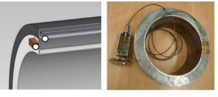
Figure 5: Alternative shielding geometry with axial meanders (left), the SQUID, housed in the little brown box, is connected between the two marked dots. Right: prototype of the Axial CCC made from Lead with attached SQUID electronics.
