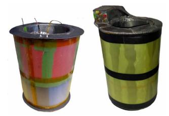
Figure 7: DCCC prototype, built from lead with diameter 300 mm and length 600 mm. Left: Pickup coils #1 and #2 mounted to the inner cylinder of the shielding (covered with tape). Right: DCCC completed and closed, with the outer meander shielding and the SQUID housing.
