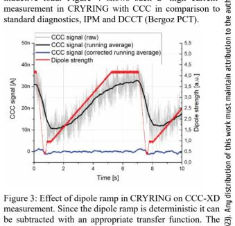
be subtracted with an appropriate transfer function. The 1.4 Hz pertubation from the cryostat pulse tube cooler, visible on the raw signal, was eliminated by a software bandblock filter (1-3 Hz) [9].
