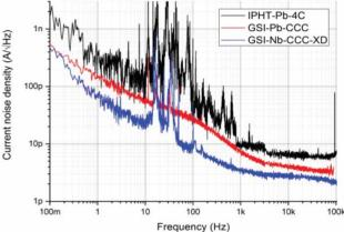
Figure 6: Noise spectra measured at the FAIR CCC-XD (blue), the GSI prototype from [3] (red) and one of the first prototypes of the axial CCC, shown in Fig. 5.
