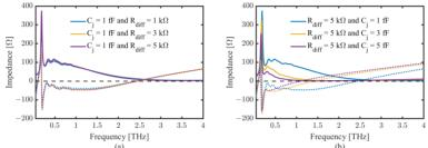
Figure 3: (a) Total device impedance for constant  $C_i = 1$  fF and variable  $R_{diff}$ , (b) Total device impedance for variable  $C_i$ and constant  $R_{diff} = 5 k\Omega$  with SLSA antenna with  $2.4 \times 2.4 \mu m^2$  channel. Dotted lines: imaginary part, solid lines: real part of impedance, on substrate of 4.5  $\mu$ m thickness and dielectric constant of  $|\varepsilon_r| = 2.8$ .
