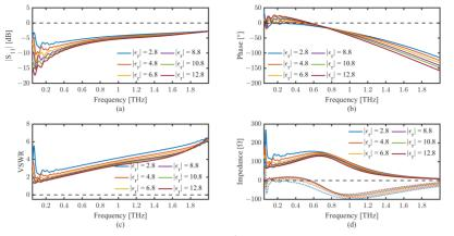
Figure 2: Effect of variable  $|\varepsilon_r|$  on LSA antenna with  $10 \times 8 \,\mu\text{m}^2$  channel with ZBSD having  $C_j = 1$  fF and  $R_{diff} = 5 \,k\Omega$ , (a)  $|S_{11}|$ , (b) Phase response, (c) VSWR response and (d) Impedance, solid lines represent real part and dotted lines represent imaginary part.
