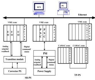
Figure 1: Control architecture for BII power supplies.
