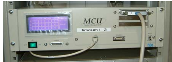
Figure 3: The MCU for pulse motor control.
