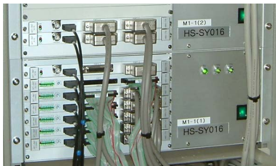
Figure 2: The remote boards of OPT-VME.
