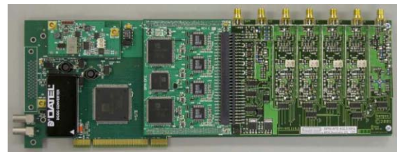
Figure 3: SNS BPM PCI card. Digitizers are in the center, downconversion mixers and filters are to the right.
