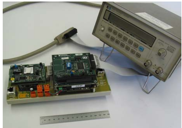
Figure 1: The GPIB Appliance: PC/104 CPU with GPIB interface mounted on TRIUMF backplane.
