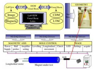
Figure 3: Measuring system architecture
