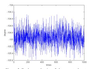
Figure 5: Background noise of phase control system Firstly, we tested the background noise of phase control system in LINAC operation condition. In the test, RF
