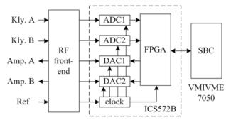
Figure 2: Layout of phase control system
