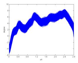
Figure 6: Interpulse phase shift of klystron forward signal
