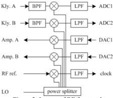
Figure 3: Layout of RF front-end
