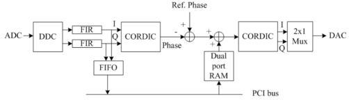
Figure 4: Layout of one channel in FPGA
