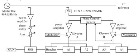
Figure 1:The layout of SSRF LINAC
