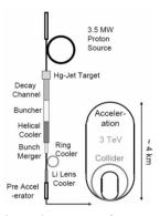
Figure 8: Layout of a Muon Collider
