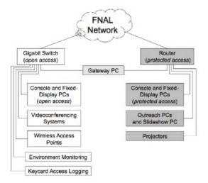
Figure 3: LHC@FNAL Computing Network.
