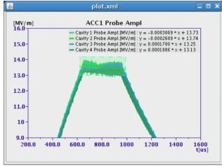
Figure 2: The plot component with a linear fit.
