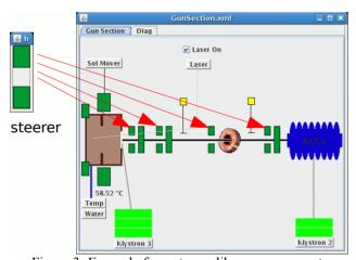
Figure 3: Example for a steerer library component.
