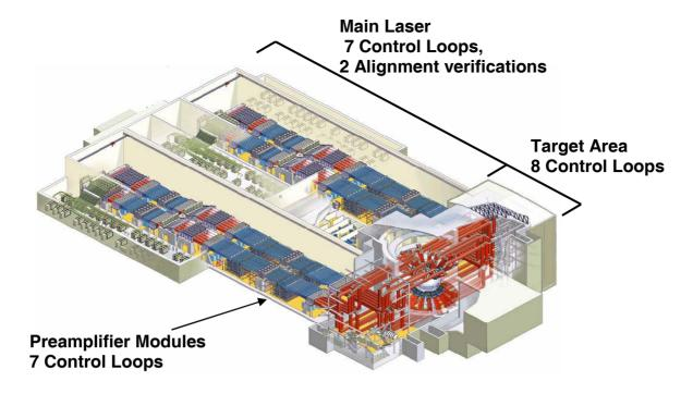
Figure 1: The National Ignition Facility incorporates 3,800 closed-loop alignment operations.
