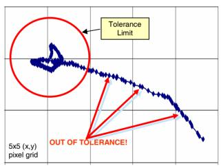
Figure 8: Example demonstrates required sub-pixel accuracy was not met because of high uncertainty.
