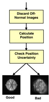
Figure 6: General algorithm block diagram.
