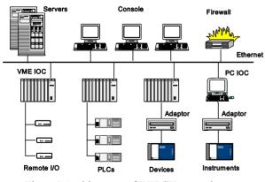
Figure1 Architecture of BEPCII control system.
