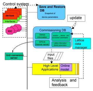
Figure 1: Interrelation of components in the commissioning software system.
