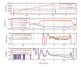
Figure 7: RF amplitude and phase waveform before and after correction with bunch train 600 nsec beam, both amplitude and phase are corrected simultaneously.
