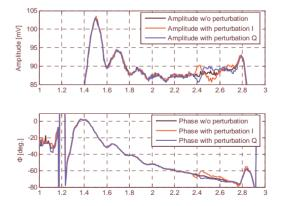
Figure 4: RF amplitude and phase response measurement, the perturbation is applied to I channel (red curve) and the perturbation is applied to Q channel (blue curve). This measurement is without beam.
