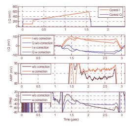
Figure 5: RF amplitude and phase waveform before and after correction I signal without beam, flatness of amplitude and phase are improved.
