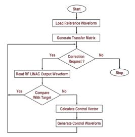
Figure 3: Flow chart of the feed-forward correction.
