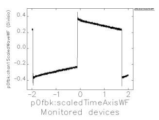
Figure 3: Response of FPGA output with step-function drive.
