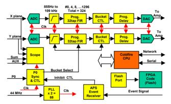
Figure 2: FPGA block diagram of P0 Feedback.
