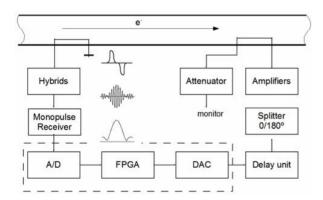
Figure 1: Block diagram of the feedback system.
