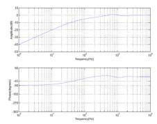
Figure 5: Amplitude and phase response of the sensitivity function.
