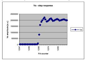
Figure 2: Libera Fast acquisition response, with a sampling rate of 10 kHz.
