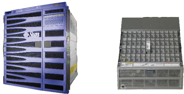
Figure 1: The DAQ core system is build up of two SUN enterprise machines – one hosting 32 GB main memory, the so called buffer manager - the second (used for storing the data of the last weeks) hosting 22 TB disc space.
