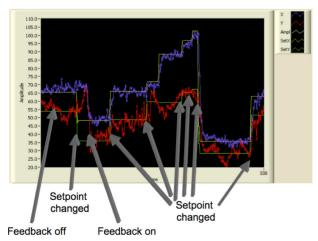
Figure 3. Measured positions and setpoints while adjusting the setpoints.
