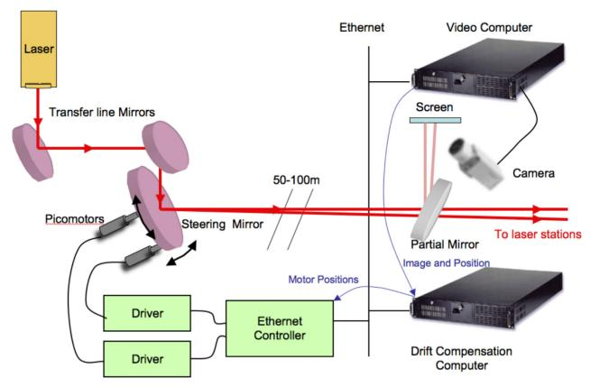
Figure 1. Diagram of the Drift Compensation System.
