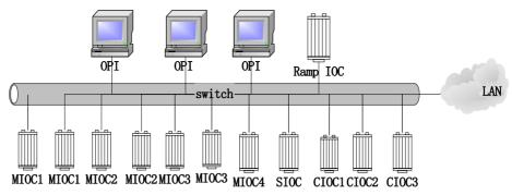
Figure 3: PS IOC Distribution in the network.
