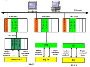
Figure 1: BEPCII PS control system architecture.
