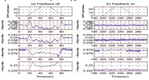
Figure 1: Effectiveness of the orbit feedback loop versus phase change of the EPU5.6 undulator. (a) without feedback; (b) with feedback
