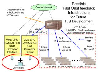
Figure 7: Architecture of the proposed orbit feedback system for further upgrade for TLS.
