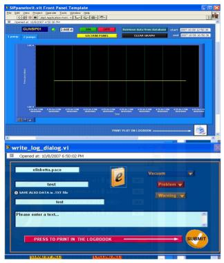
Figure 6: LabVIEW control panel for creating an entry in SPARCbook.
